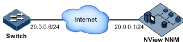
Figure 10-12 Hardware environment monitoring networking
